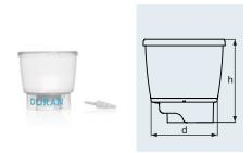
Designed for sterilization or clarification of aqueous cell culture media Supplied as a filter funnel unit for use with the DURAN\* TILT bottle (with GL 45 thread adaptor) or 45 mm media bottles. Comes in three different asymmetric pore sizes (0.1  $\mu$ m, 0.2  $\mu$ m, or 0.45  $\mu$ m). Raised moulded graduation marks for easy volume reading. Manufactured in a Class 100,000 clean room from Class VI, non-cytotoxic materials. Supplied sterile.
