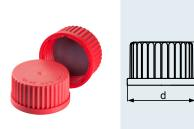
High leak tightness through use of PTFE coated silicone seal (peroxide-cured silicone). More chemically and heat resistant than PP screw cap. A matching ETFE pouring ring is also available, permitting clean, drip-free use.
