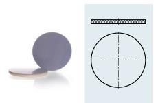
Suitable for PBT screw caps and tamper-evident screw caps. Heat resistance:  $130\,^{\circ}$ C (vapour) and  $200\,^{\circ}$ C (dry heat). Good chemical resistance due to PTFE coating. Silicon is peroxide-cured.
