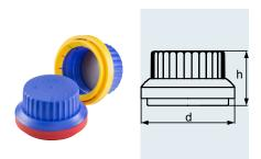
The tamper-evident screw caps are available with either a plug seal or a PTFE faced silicone cap liner (peroxide cured silicone). The integral coloured plastic ring tears when the cap is first opened, and is retained on the bottle neck. Therefore it can be clearly seen if the bottle has been opened after being first sealed. After the initial removal, both caps will still function as "normal" screw cap.
